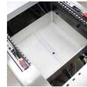
Auto-Slide Tooling System. Available with the Mammoth® is an innovative pneumatic auto-slide tooling system for faster and safer tool changes.
