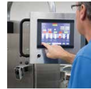
Simple Touchscreen Operation. All safety & operation functions are built into touchscreen.
