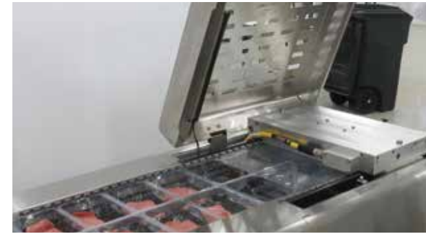
Hinged Lid: Gives easy access for fast die change outs.
