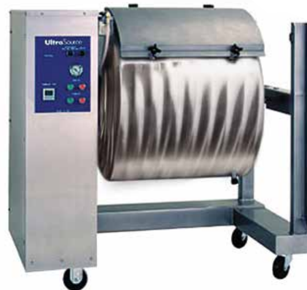
LT-30 Vacuum Tumbler 400-lbs. Working Capacity
