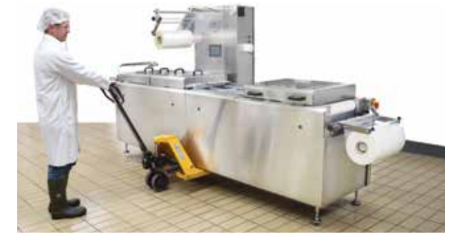
Move Easily — with a pallet jack or forklift.
