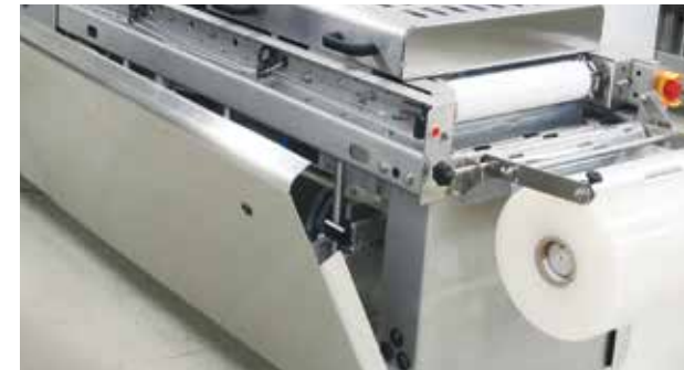
Side Panels: Easily removed or tilt away for access to components & easy wash down.
