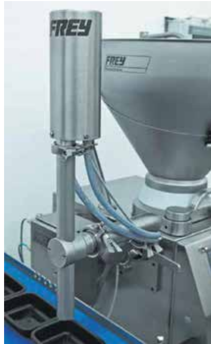
DK40 DK40 pneumatically driven dosing piston for vertical filling of cans, trays & other receptacles. Adjustable volume control with initial diameter of 40 mm.
