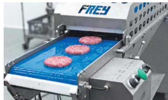
Automatic Burger Patty Line (DMFB 92) Diversify your product mix by adding a portioner & former & a paper interleaver with an integrated tray dispenser to your stuffer for creating hamburger patties.
