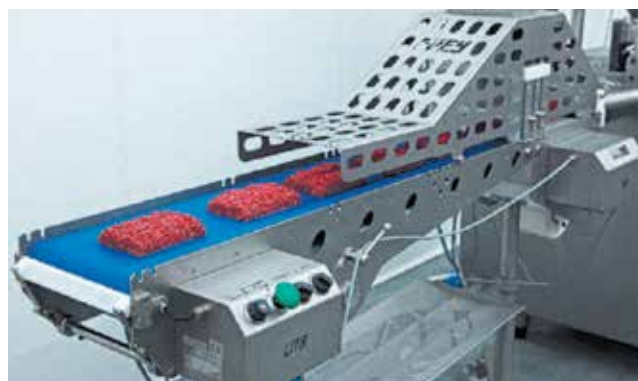
CLPS320 Portioner Ideal for large production of ground meat, the CLPS320 portions & cuts the product with or without paper.
