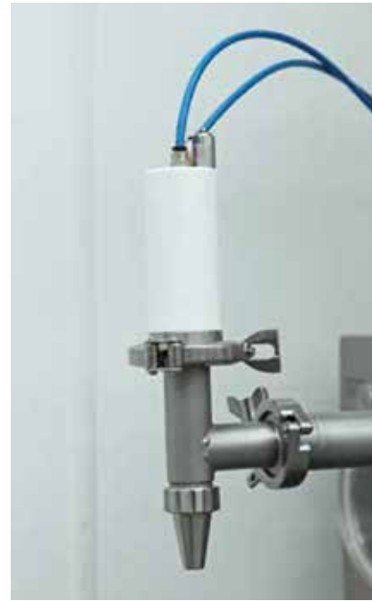
DK20S DK20S dosing unit fixed to the filling stuffer with adjustable portion volume. 20 mm initial diameter. Compressed air necessary.
