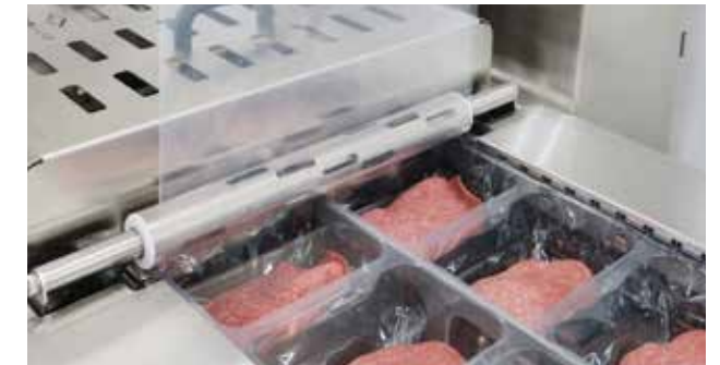
Hygienic Rollers: Slotted to allow easy wash down draining.
